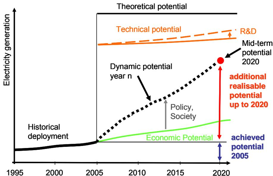
Figure 2.1. Methodology for the definition of different potentials
