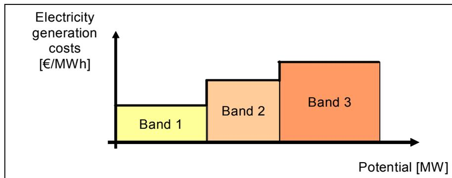
Figure 2.2. Relation between costs and potential for one technology
