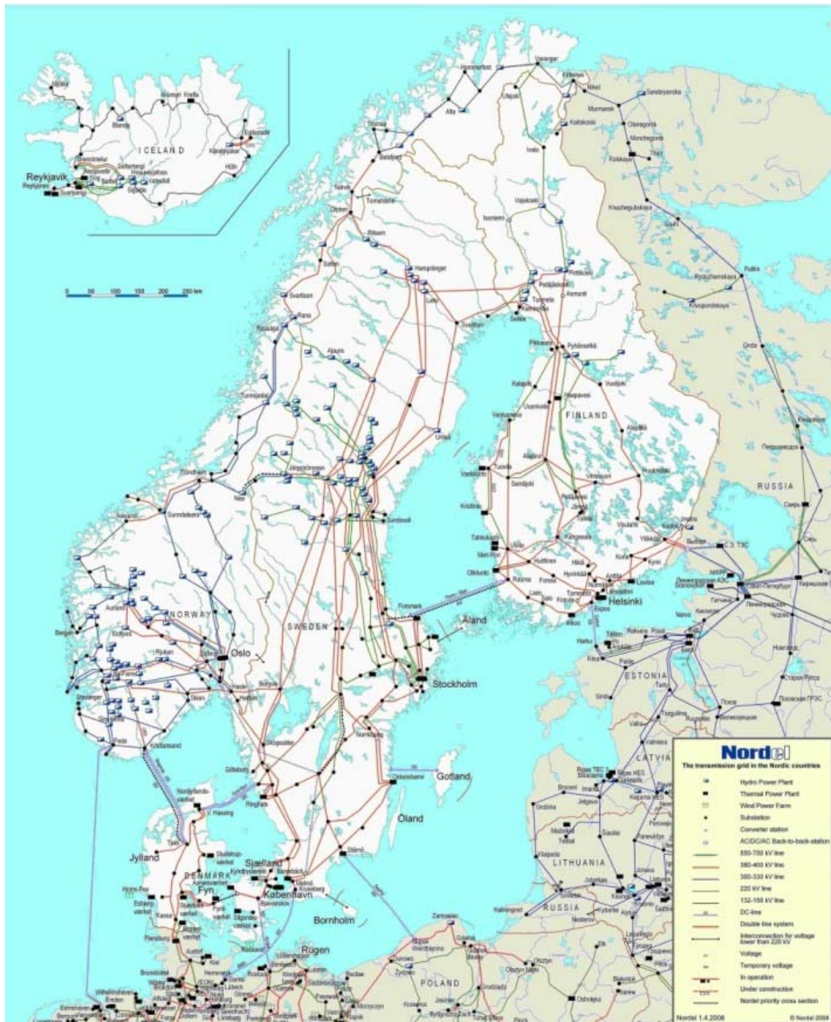
Figure H-2: The transmission grid in the Nordic countries (figure is copied from Nordel's web-site).
