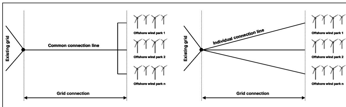
Figure 2.2. Illustration of the term grid connection as used in **GreenNet-EU27** for the case of an individual connection of offshore wind farms to the existing onshore power grid (right) and coordinated connection of offshore wind farms via a common link (left)
